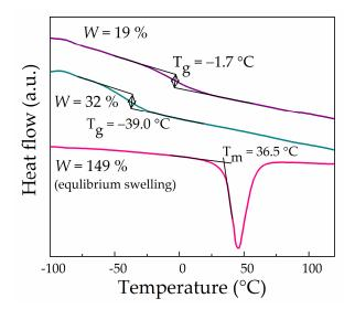
Figure 7. DSC curves for Li-Nafion with different contents of EC (40 °C/min).
