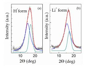
**Figure 5.** Wide-angle diffraction pattern of "dry" Nafion 115 membrane before (**a**) and after (**b**) lithiation.
