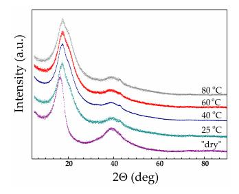
**Figure 8.** Wide-angle X-ray diffraction patterns for "dry" Li-Nafion and membrane samples swelled with EC/SL mixture with  $\omega$ (SL) = 0.2 at different mixing temperatures specified in the figure.
