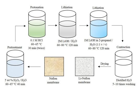
Figure 2. Scheme of the Nafion membrane lithiation process.
