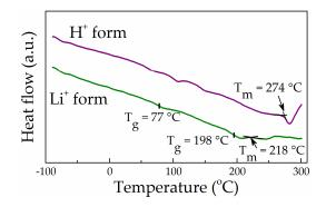
**Figure 6.** Differential scanning calorimetry (DSC) curves for the "dry" samples of Nafion 115 in H<sup>+</sup> and Li<sup>+</sup> forms.
