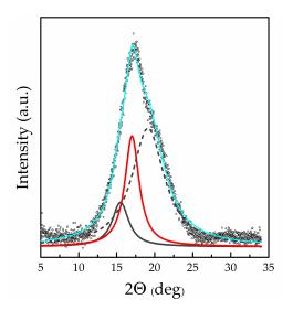
**Figure 9.** Decomposition of X-ray diffraction profile near (100) Bregg peak for Li-Nafion saturated with EC/SL mixture with  $\omega$ (SL) = 0.2 at the mixing temperature of 25 °C.
