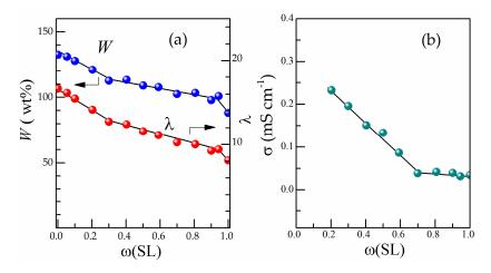
**Figure 3.** Weight uptake (*W*) and molar uptake ( $\lambda$ ) (**a**) and conductivity of swollen Li-Nafion membrane at 25 °C (**b**) as a function of  $\omega$ (SL) (mixing temperature of 40 °C).
