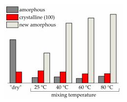
**Figure 10.** Amorphous and crystalline peak areas for Li-Nafion samples before and after swelling with an EC/SL mixture with  $\omega$ (SL) = 0.2 at different mixing temperatures (specified in the diagram).
