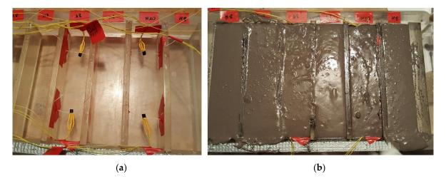
**Figure 2.** The measurement of temperature changes in samples during the curing process: (**a**) thermometers inside the empty molds; (**b**) fresh geopolymer mixture inside the molds.
