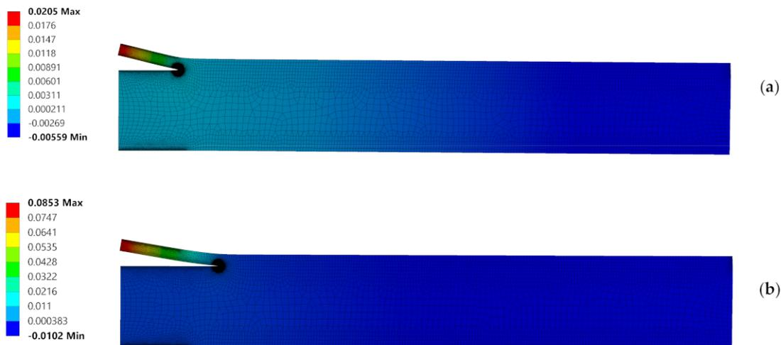
Figure 11. Effect of void in deamination growth (mm) (a) Delamination growth in single voids case, (b) Delamination growth due to additional voids.
