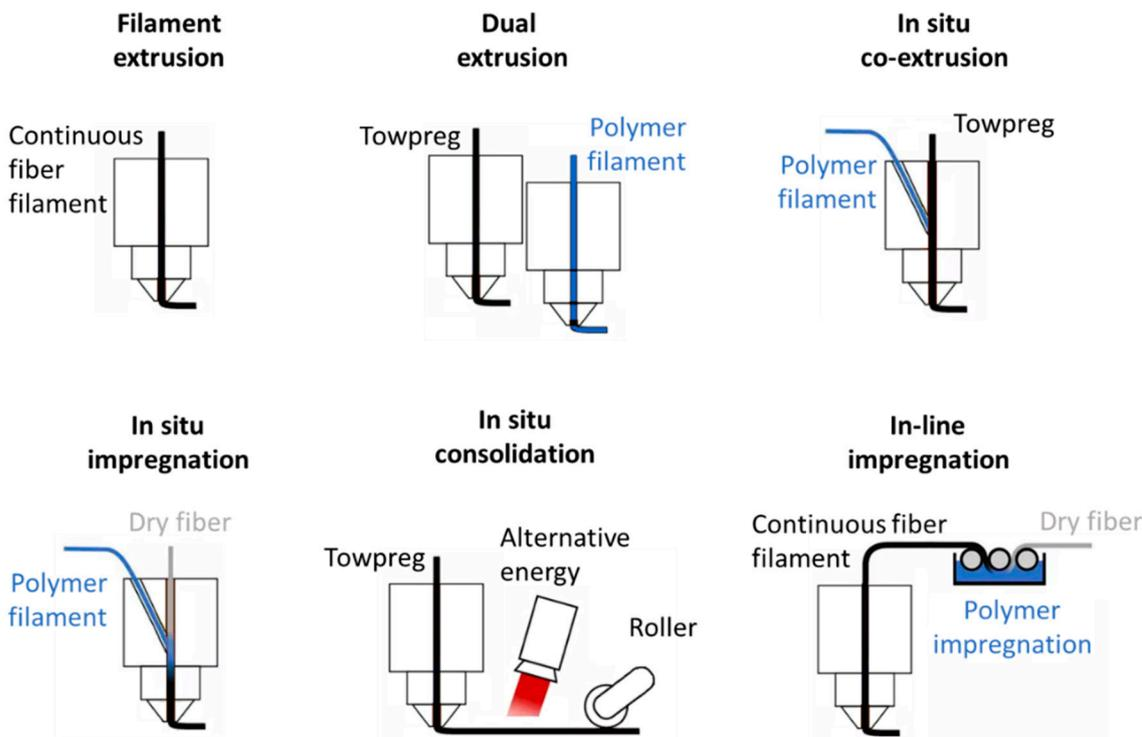
**Figure 18.** Main commercial of FFF processes for CFRTPC printing classified by increasing complexity, inspired by [116].
