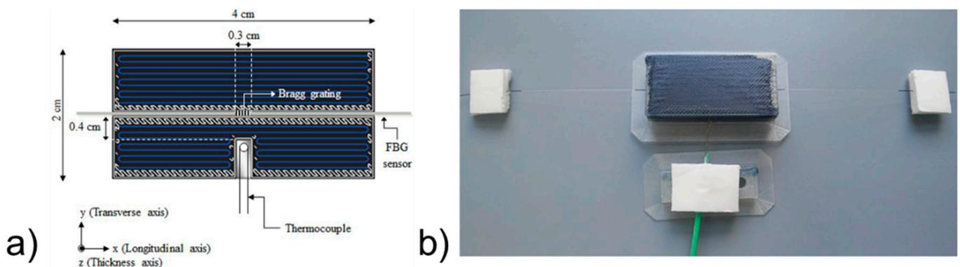
**Figure 8.** (a) Schematic of the midplane of a  $0^\circ$  fiber reinforcement orientation of a 3D printed CFRTPC with the location of the FBG sensor and the thermocouple, and (b) picture of a 3D printed CFRTPC specimen containing an embedded FBG sensor and a thermocouple [71] (copyright (2019), with permission from Elsevier).
