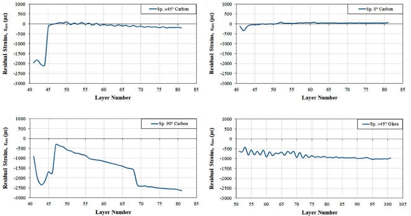
**Figure 9.** Effect of 3D printed CFRTPC’s fiber orientation and type on process-generated residual strains [71] (copyright (2019), with permission from Elsevier).
