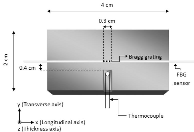
**Figure 10.** Schematic of a 3D printed neat TP with the location of the FBG sensor and the thermocouple [72] (copyright (2016), with permission from Elsevier).
