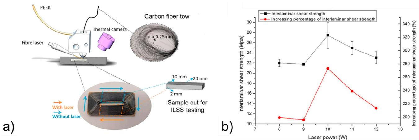
**Figure 6.** Laser-assisted printing process [21]: (a) diagram of the preparation of continuous CF/PEEK composite samples for ILSS testing and (b) ILSS and increasing percentage of ILSS with different laser powers (copyright (2019) with permission from Elsevier).
