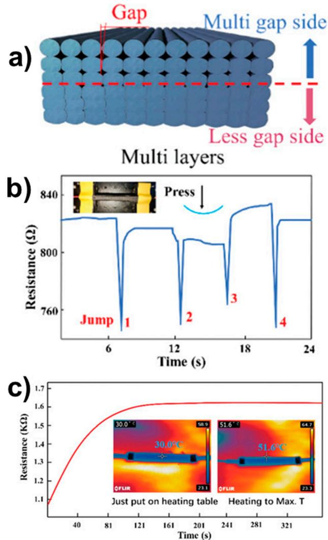
**Figure 12.** Self-sensing technology to detect strain and temperature variation in 3D printed PLA/carbon black composite: (a) material design showing gaps, (b) resistance variation when the composite is subjected to compression, and (c) resistance variation when the composite is subjected to a temperature increase from 30 °C to 52.6 °C [91] (copyright (2020), with permission from Wiley-VCH Verlag GmbH & Co).
