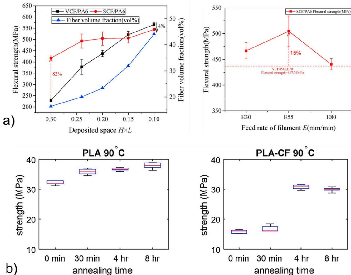
**Figure 5.** (a) Effect of printing parameters, sizing, and fiber fraction on the mechanical strength of 3D printed PA composite [19] (copyright (2018), with permission from Elsevier) and (b) effect of annealing on the mechanical strength of 3D printed PLA [20] (copyright (2019), with permission from Elsevier).
