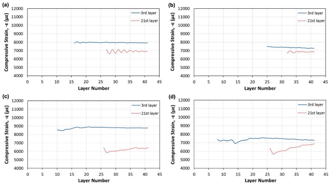
**Figure 11.** In situ measurements of the compressive strain of 3D printed neat TP as a function of layer number for horizontally (a,b) and perpendicularly (c,d) positioned specimens on the print bed, where the FBG sensors are longitudinally or transversely embedded, respectively [72] (copyright (2016), with permission from Elsevier).
