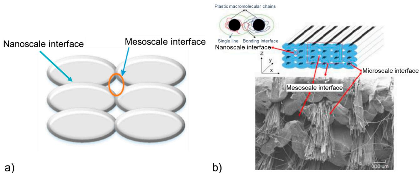
**Figure 1.** Multiscale interfaces in 3D printed (a) neat TPs [5] and (b) CFRTPCs [10] (copyright (2017), with permission from Emerald Publishing Limited). Nanoscale and mesoscale interfaces are generated between two and four printing lines, respectively, and microscale interfaces are generated between the TP matrix and the fiber bundle.
