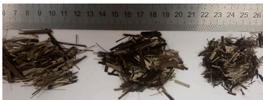
Figure 2. Three types of the chopped basalt fibers (CBFs) with different fiber lengths used in this work, from left to right: the fiber length of 24 mm (24 mm CBFs), the fiber length of 12 mm (12 mm CBFs), the fiber length of 6 mm (6 mm CBFs).
