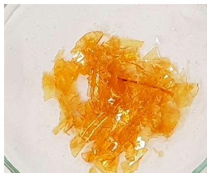
**Figure S3.** Images of bromide-form S29QA30-C6 membrane fragments.
