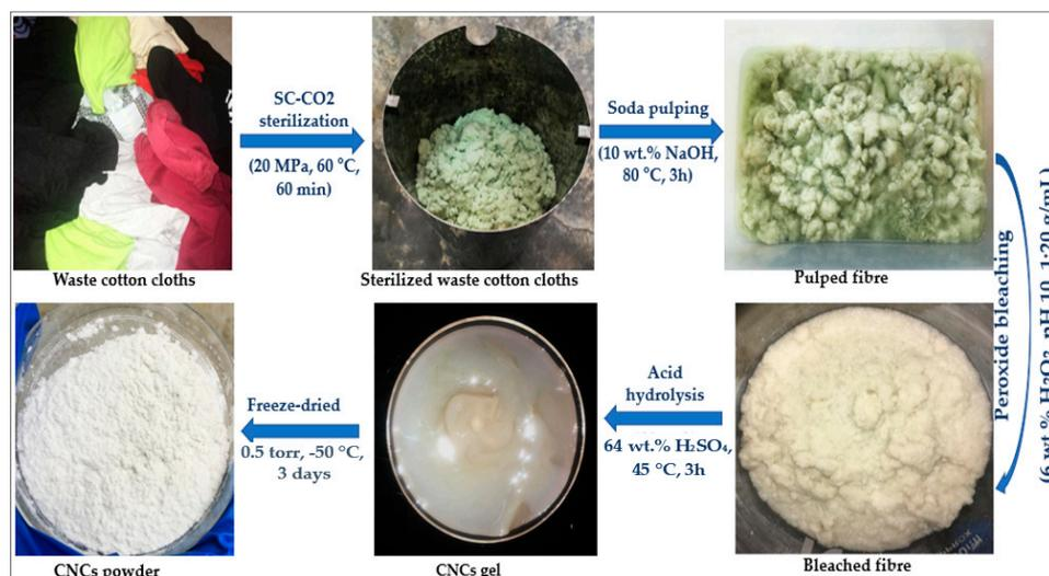
**Figure 1.** Schematic diagram for the isolation of cellulose nanocrystals (CNCs) from waste cotton cloths.
