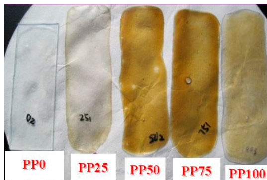
Figure 5. Appearance of the coatings immersed in seawater for 30 days
