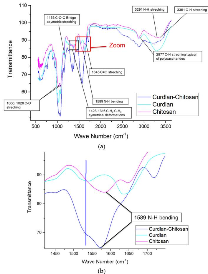
**Figure 3.** ATR-FTIR spectra of curdlan and chitosan starting polymers and of the curdlan–chitosan fibers. (a) The full spectrum with peaks attribution [51]. (b) Zoom on the 1400 to 1700  $\text{cm}^{-1}$  spectral range to identify characteristic peaks of both curdlan and chitosan of the blend spectrum (blue line denotes the 1530  $\text{cm}^{-1}$  band specific to curdlan).
