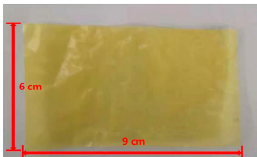
Figure S1. Optical photograph of PI@SPFEK composite membrane.
