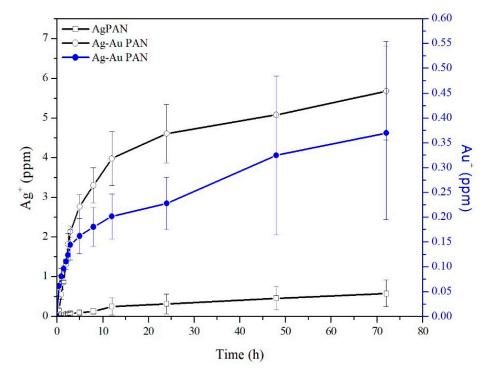
Figure 3. Profile of silver ion release curve.
