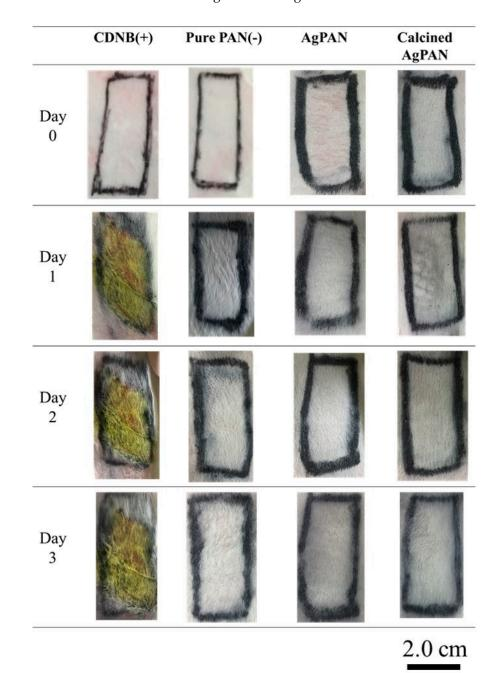
Figure 6. Testing for sensitivity of animal skin to various types of nonwoven mats for 3 days.
