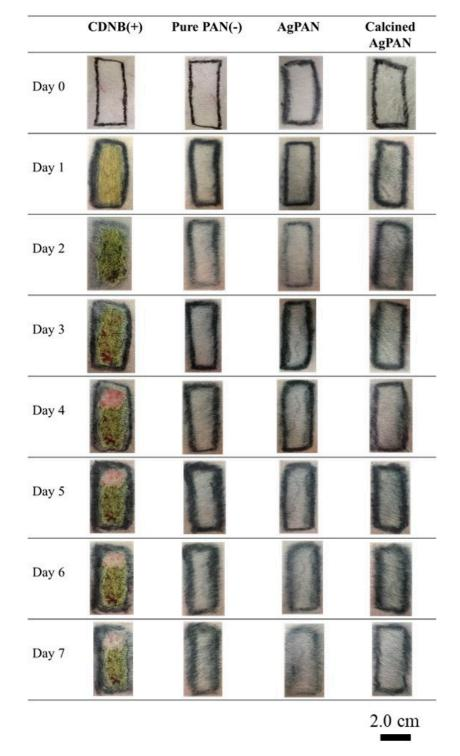
Figure 7. Testing for irritation of animal skin by various types of nonwoven mats for 7 days.
