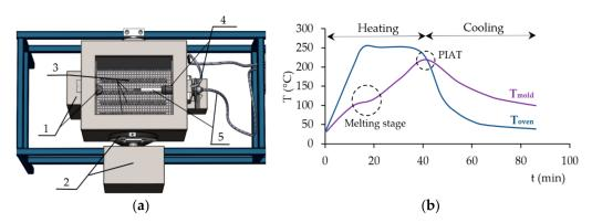
**Figure 2.** (a) A description of rotomolding machine 1—first stepper motor, 2—a belt drive with second stepper motor, 3—heaters, 4—temperature sensor in the oven, 5—temperature sensor in the mold; (b) typical curve plotted during the process.
