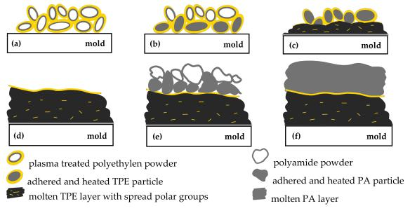
Figure 7. The TPE and PA layer built-up in multilayer rotational molding.
