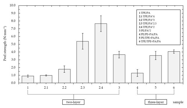
Figure 3. Comparison of peel strength of various samples.
