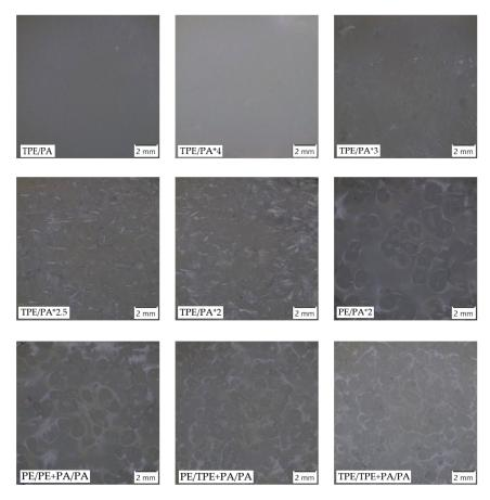
**Figure 5.** Micrographs of fracture surfaces.
