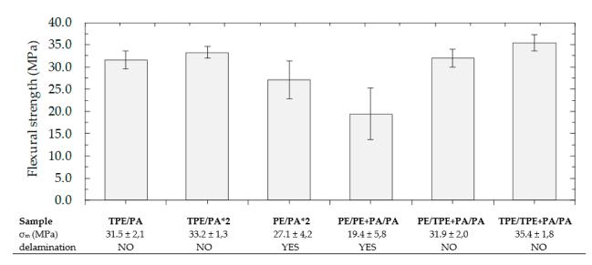
Figure 4. Results obtained from the bending test.
