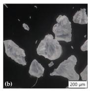
Figure 1. Micrographs of used powders (a) polyethylene; (b) polyamide.
