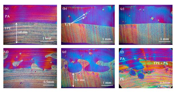
**Figure 6.** Pictures of cross-sections in polarized microscopy (a) plasma-treated polyethylene (TPE)/polyamide (PA); (b) TPE/PA\*4; (c) TPE/PA\*3; (d) TPE/PA\*2.5, (e) TPE/PA\*2; (f) PE/TPE + PA/PA.
