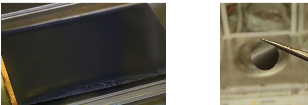
Figure 2. Polymer electrolyte layer on graphite electrode directly after polymerization ( left ) as well as a punched-out membrane on a \text{LiNi}_{1/3}\text{Mn}_{1/3}\text{Co}_{1/3}\text{O}_2 electrode for tests in a coin cell ( right ).
