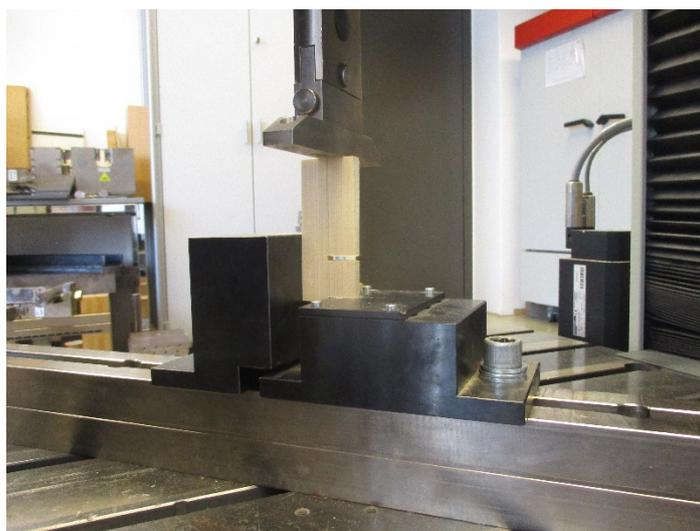
**Figure 6.** Shear strength test of the single-layer solid spruce laminated timber.
