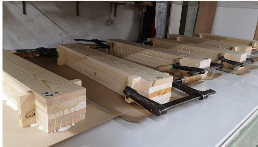
**Figure 5.** Production of the spruce laminated timber blocks (5 × 20 × 120 × 750 mm) in the cold process before pressing.
