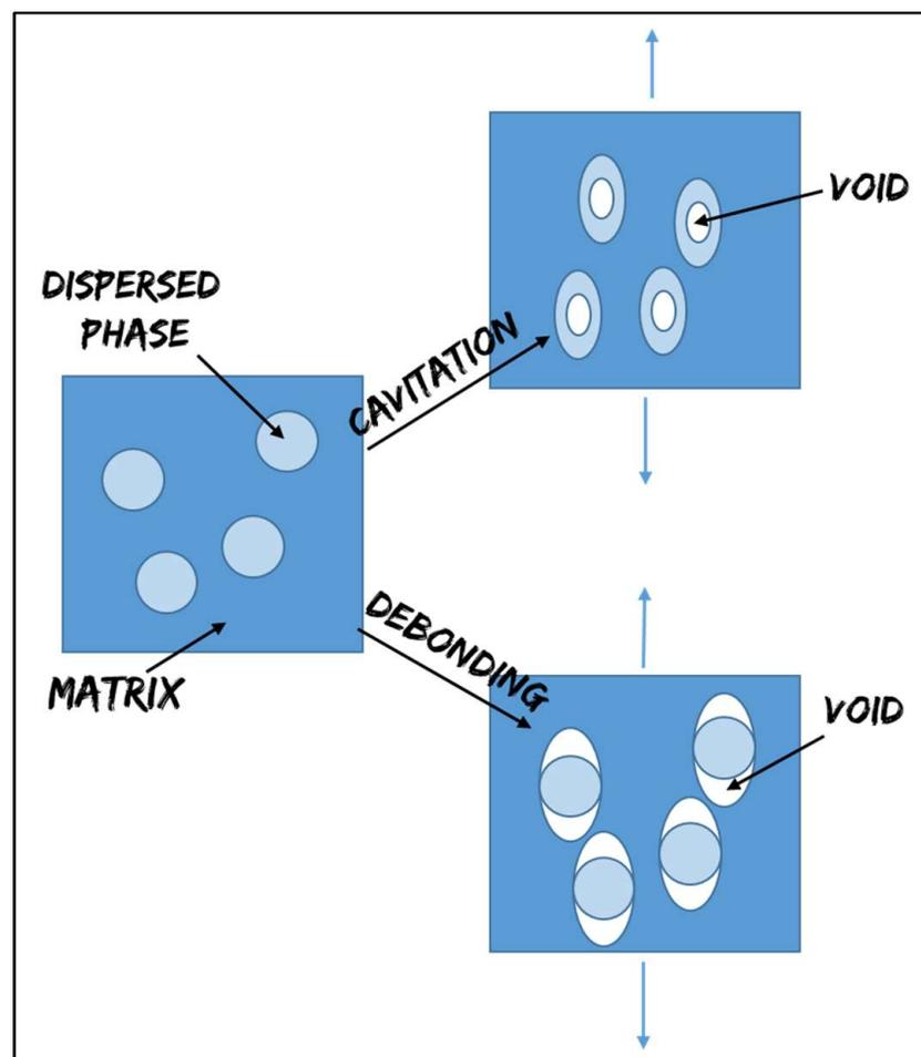
**Figure 1.** Cavitation and debonding mechanisms.
