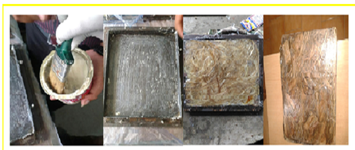
Figure 4. The fabrication process of the hybrid epoxy composite.
