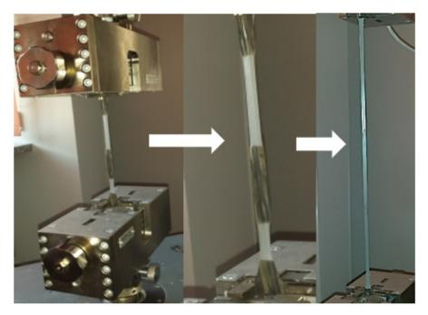
Figure 7. View of the sample during tensile test.
