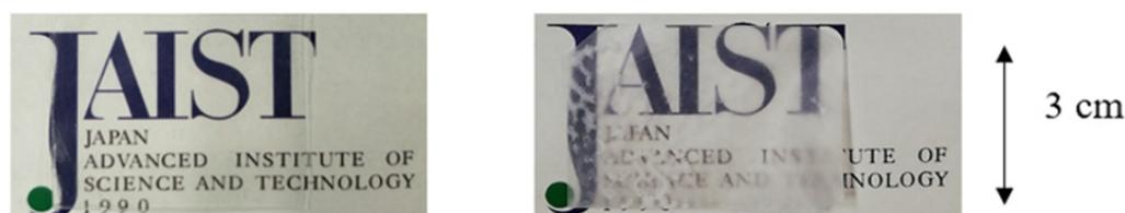
**Figure 2.** Photographs of the films with 200  $\mu\text{m}$  thickness: PVA/ $\text{Mg}(\text{ClO}_4)_2$  (**left**) and PVA/ $\text{MgSO}_4$  (**right**). Each film had a salt content of 0.05 as a molar ratio relative to the quantity of PVA hydroxyl groups.
