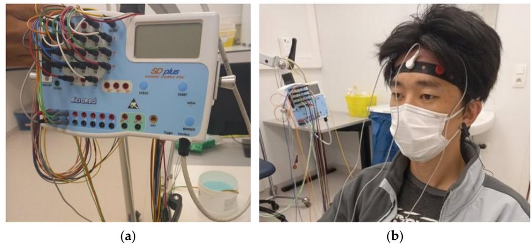
**Figure 12.** Electroencephalography (EEG) measurement: (a) Brain Quick EEG Clinical line and (b) photographic image of actual EEG measurement.
