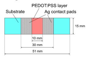
Figure 1. Layout of tested samples.
