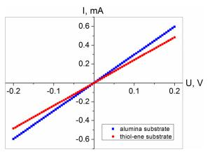
Figure 4. Characteristic current-voltage curves of PEDOT:PSS films on alumina and thiol-ene substrates.
