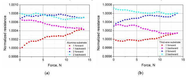
**Figure 9.** Dependence of the normalized resistance of PEDOT:PSS films on the applied force during the first two cycles of loading: (a) alumina substrate and (b) thiol—ene substrate on alumina. The notation "forward" means an increase in force, while "backward" means a decrease.
