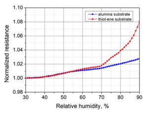
**Figure 13.** Normalized resistance of PEDOT:PSS films on alumina and thiol—ene substrates versus relative humidity.
