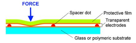
Figure 8. Design of a resistive touch screen.
