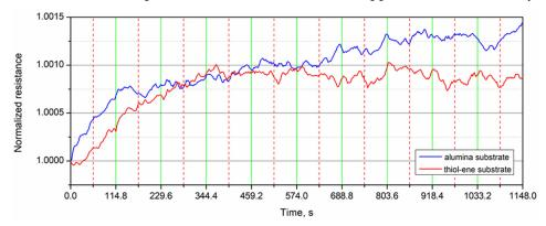
**Figure 10.** Normalized resistance of the PEDOT:PSS films versus time over 10 cycles of applied strain. The vertical dashed red lines correspond to the maximum load and the solid green lines correspond to zero load.
