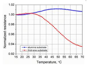
**Figure 12.** Normalized resistance of PEDOT:PSS films on alumina and thiol–ene substrates versus temperature.
