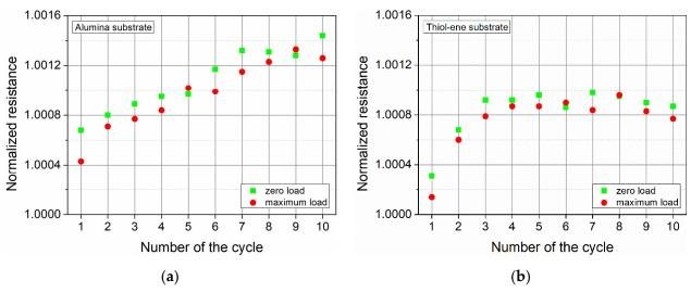
**Figure 11.** Normalized resistance of the PEDOT:PSS films at zero and maximum load versus the number of load–unload cycles: (a) alumina substrate and (b) thiol–ene substrate on alumina.
