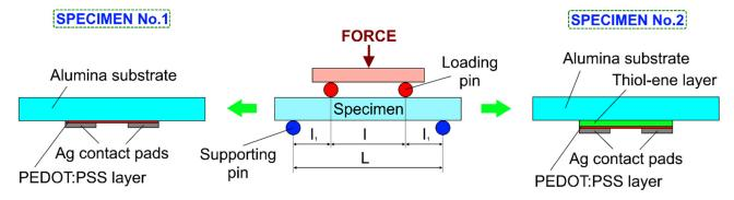
**Figure 2.** Four-point bending test setup.
