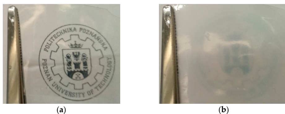
Figure 7. Pictures of materials obtained by the photopolymerization of the composition containing equilibrium mixture of monomers with 50 wt.% of NMP (5Ex:5HP_50) (a) after polymerization, (b) after electrolyte sorption.
