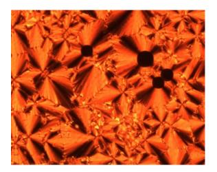
Figure 7. Focal-conic textured smectic A liquid crystalline phase present in compound 30c [42].
