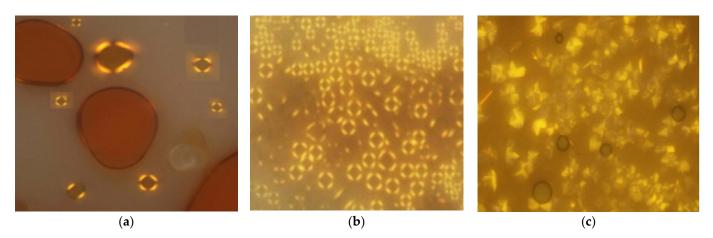
**Figure 6.** Polarizing micrograph ring-like texture of (**a**) compound **29**a at 123.0 °C, (**b**) compound **29**b at 191.0 °C, and (**c**) cone-like texture of hexatic phase of compound **29**c at 123.0 °C [41].
