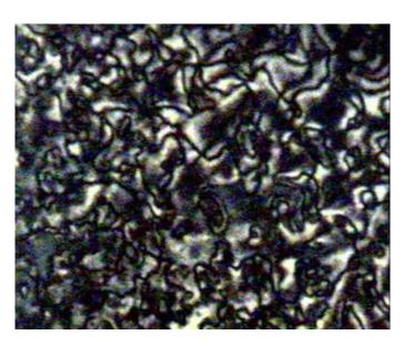
Figure 2. Optical texture of compound 11a at 210.0 °C [25].
