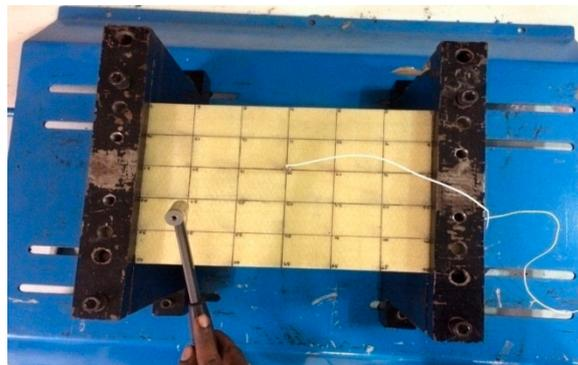
**Figure 4.** Experimental setup for the CFCF boundary condition.
