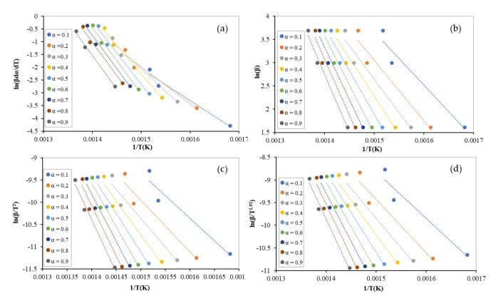
**Figure 3.** Linear regression lines of binary equi-mass PP and PS mixtures at different conversions by: (a) Freidman; (b) FWO; (c) KAS; and (d) Starink.
