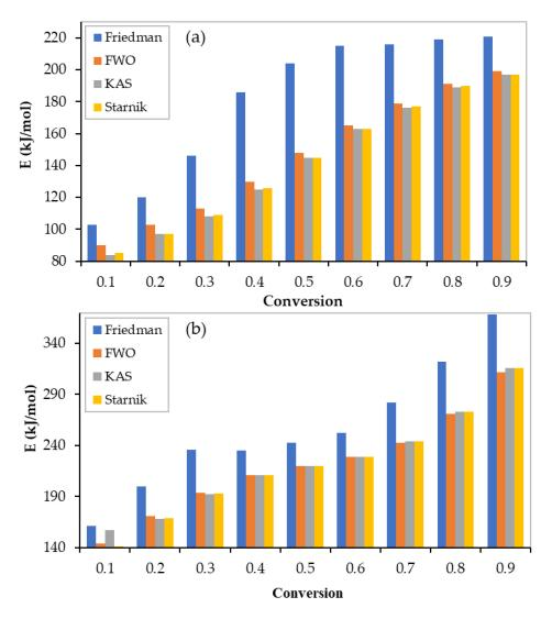
**Figure 5.** Activation energies obtained by different model-free models: (a) binary mixtures; (b) ternary mixtures.
