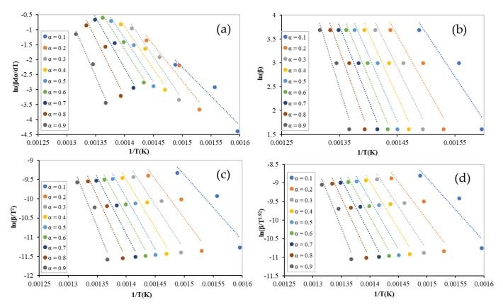
**Figure 4.** Linear regression lines of ternary equi-mass PP, PS, and LDPE mixtures at different conversions by: (a) Freidman; (b) FWO; (c) KAS; and (d) Starink.
