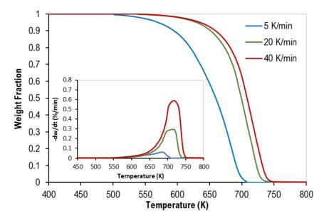
**Figure 1.** Thermogravimetric (TG) curves of equi-mass binary mixtures of PP and PS (Tests 1–3). Inset: corresponding derivative thermogravimetric (DTG) curves.
