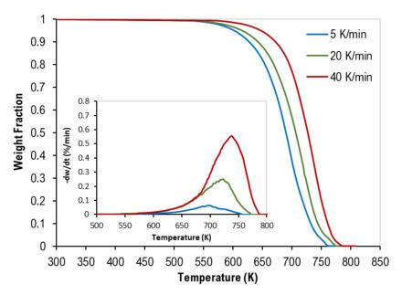
**Figure 2.** Thermogravimetric (TG) curves of equi-mass ternary mixtures of PP, PS, and LDPE (Tests 4–6). Inset: corresponding derivative thermogravimetric (DTG) curves.
