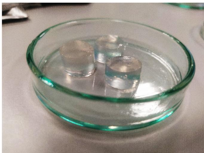
**Figure 1.** A sample photo of Coll/BG + 5%TA material, cut into a cylindrical shape for mechanical testing.
