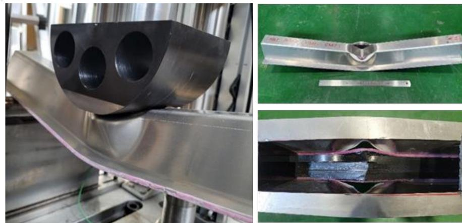
Figure 4. Failure of aluminum/CFRP component after the crash test.
