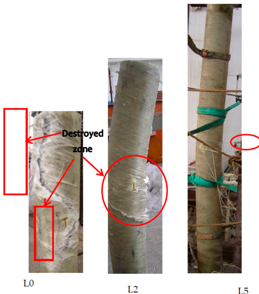
Figure 2. Typical failure modes of composite slender columns.
