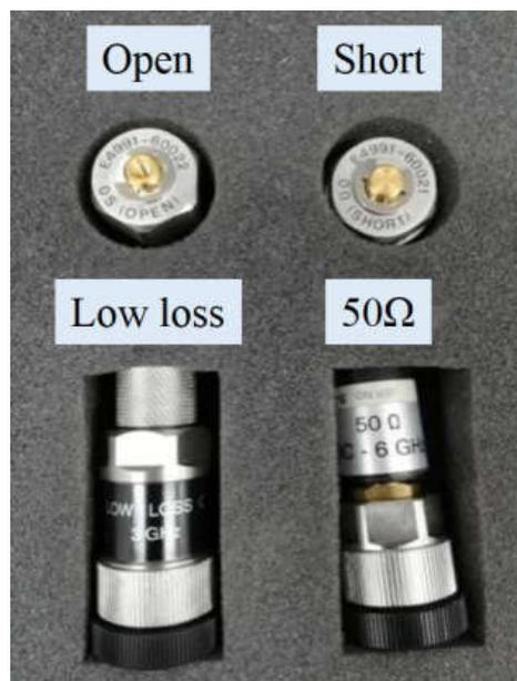
Figure 2. Four standard parts for calibration.
