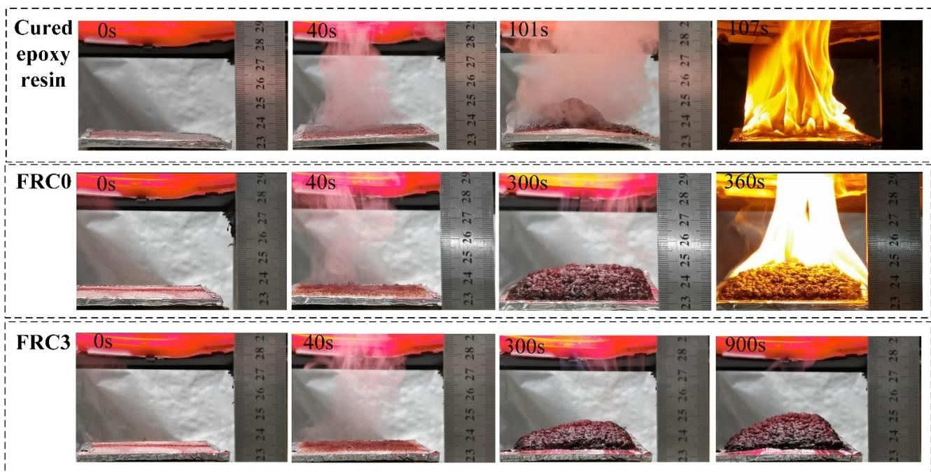
Figure 17. Digital photographs of FRC0 and FRC3 during the char layer expansion test.
