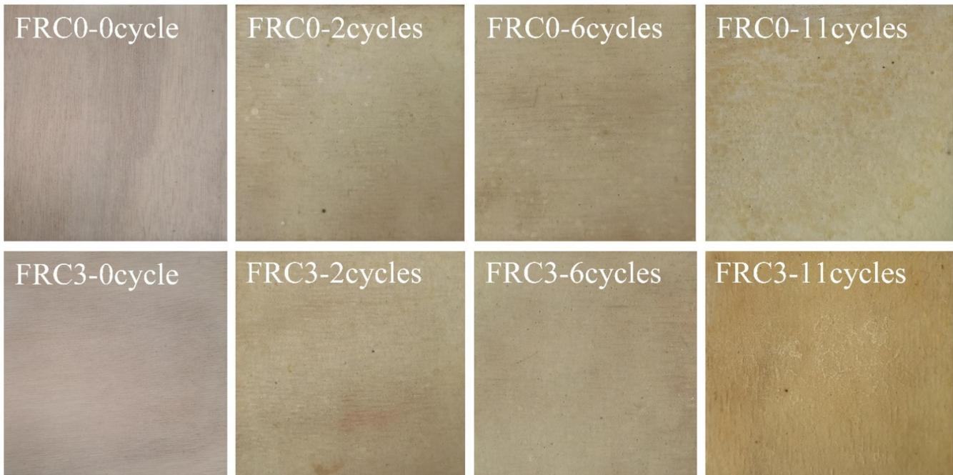
**Figure 10.** Photos of FRC0–FRC3 after different ageing cycles.
