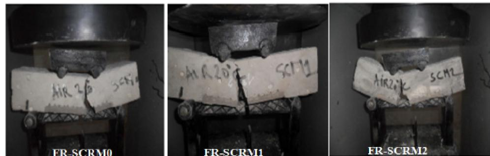
Figure 6. Breakage of specimens with fiber [112].
