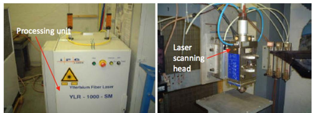
Figure 2. An IPG single-mode YLR-1000-SM 1 kW fibre laser [15].
