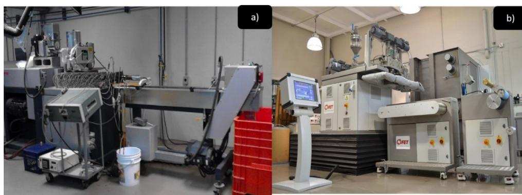
**Figure 1.** Images of extruders used in to manufacture nonwoven fabric: (a) twin-screw extruder connected to a homemade ultrasonic generator; and (b) fiber extrusion technology (FET-UK) pilot machine.
