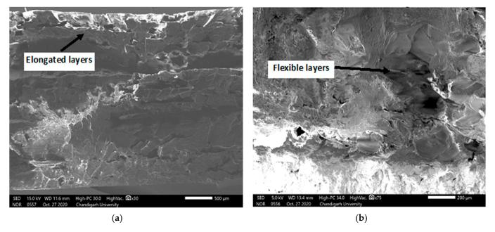
Figure 11. SEM images of point of failure of parts during (a) tensile test (b) flexural test.
