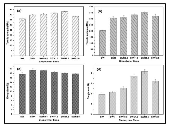
Figure 3. (a) Tensile strength and modulus (b) tensile modulus (c) elongation at break (d) toughness of seaweed, seaweed–neem, and seaweed–neem gamma irradiated film.
