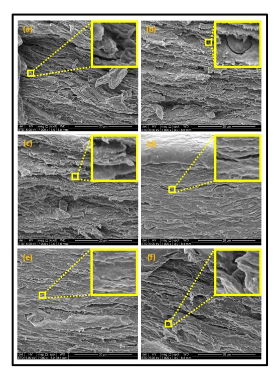
**Figure 4.** The fracture surface morphologies by Scanning Electron Microscope (SEM) of (**a**) seaweed film (control); (**b**) seaweed–neem film; (**c**) irradiated seaweed–neem at 0.5 kGy; (**d**) irradiated seaweed–neem at 1 kGy; (**e**) irradiated seaweed–neem at 1.5 kGy; (**f**) irradiated seaweed–neem at 2 kGy.
