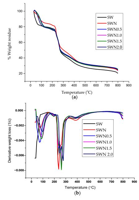
**Figure 5.** Thermal analysis indicating (**a**) TGA curve (**b**) DTG curve of the seaweed, seaweed-neem, and seaweed-neem irradiated films at different dosages.
