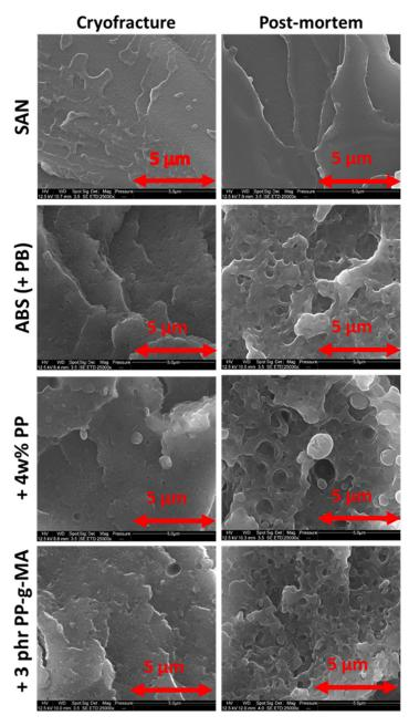
**Figure 13.** Cavitation phenomena observed on post-mortem tensile tests fragments through SEM—comparison to cryofractured samples—virgin SAN, virgin ABS, and ABS contaminated with 4 wt% PP and ABS contaminated with 4 wt% PP with 3 phr of PP-g-MA.
