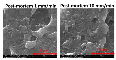
Figure 12. ABS cavitation independence toward strain speed—SEM pictures of post-mortem samples.
