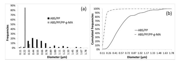
**Figure 10.** Frequencies (**a**) and cumulated frequencies (**b**) of diameters sizes distribution for ABS/PP and ABS/PP/PP-g-MA composites.
