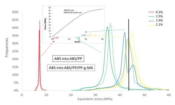
**Figure 19.** Frequencies of elements versus equivalent stresses for several macroscopic strains for ABS into ABS/PP and ABS/PP/PP-g-MA blends.
