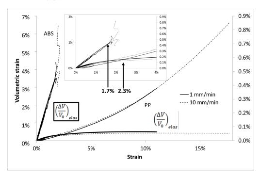
**Figure 4.** Volumetric strain vs. Lagrangian strain in uniaxial tensile tests at several imposed strain rates for ABS and PP, focus on strain until % to enhance the deviation point at 2.4% from elastic behavior for PP sample.
