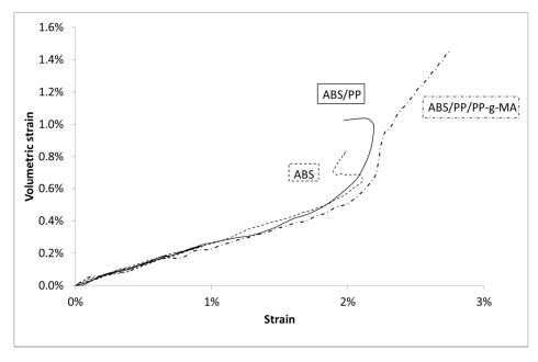
**Figure 6.** Volumetric Strain vs. Lagrangian strain in uniaxial tensile tests at 10 mm/min for ABS, PP, and composites.
