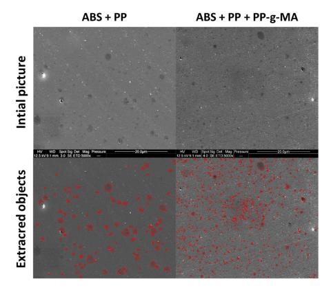
**Figure 9.** Binarization of SEM micrographs of cuts performed using an ultracyromicrotome—ABS + PP and ABS + PP + PP-g-MA systems.
