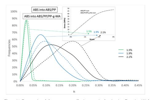
**Figure 21.** Frequencies of elements versus effective porosity fraction (see Equation (4)) for several macroscopic strains for ABS into ABS/PP and ABS/PP/PP-g-MA composites.
