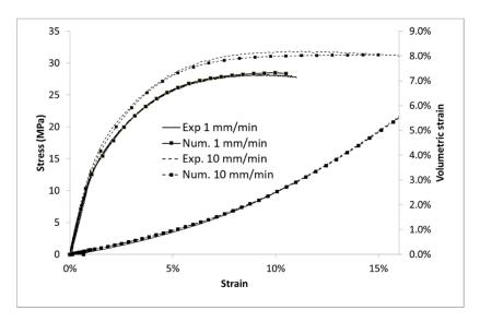
Figure 15. Modelling of PP, stress, and volumetric strain vs. Lagrangian strain.
