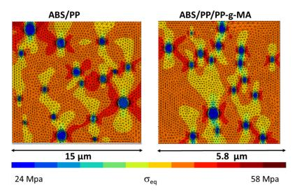
**Figure 18.** Von Mises stress cartography at 1.7% of macroscopic strain in ABS/PP and ABS/PP/PP-g-MA blends.
