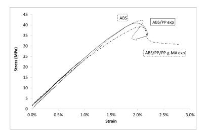
**Figure 5.** Stress vs. Lagrangian strain in uniaxial tensile tests at 10 mm/min for ABS, PP, and composites.
