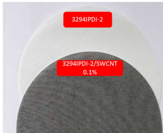
Figure 20. Appearance of UPRON fabric coated with: ( top ) 3294IPDI-2 and ( bottom ) 3294IPDI-2 dopped with 0.1 wt. % SWCNT.
