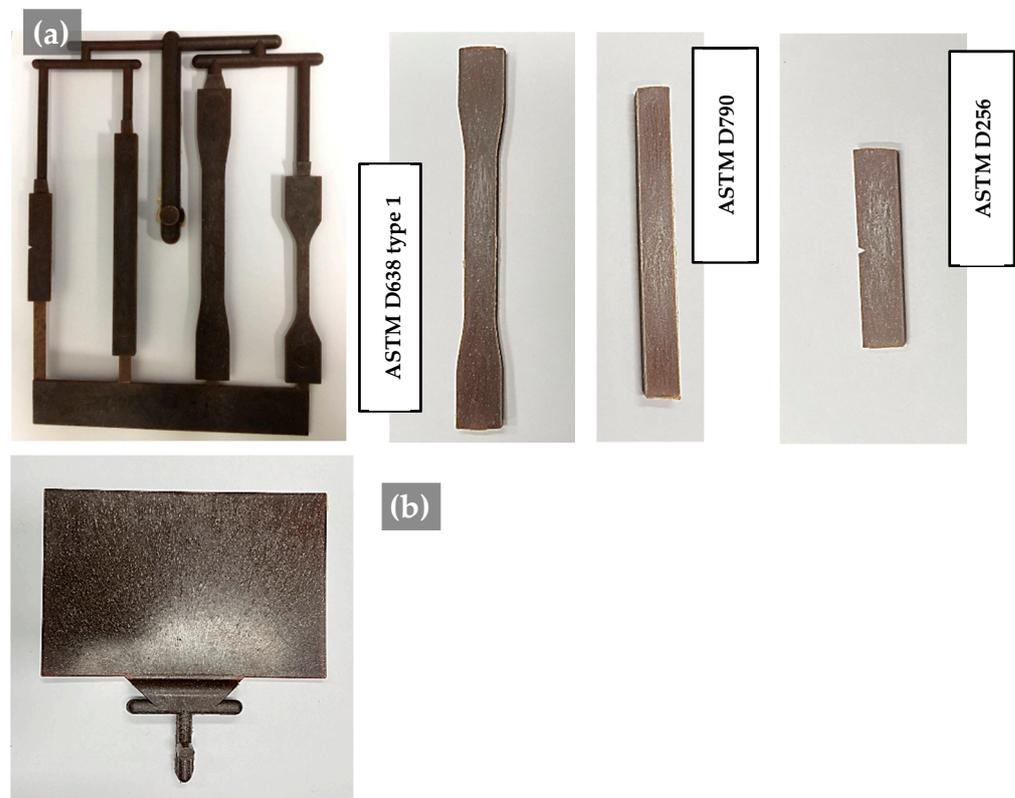
**Figure 2.** Injection-molded PP/SOC, biocomposite containing polypropylene (PP) and SOC: (a) specimen for mechanical properties evaluation; (b) specimen for SEM, XRD.
