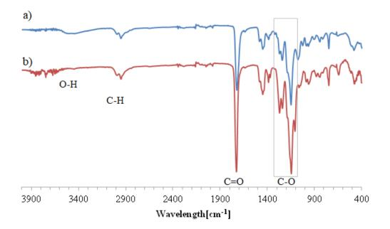
Figure S2. FT-IR spectra for (a) precursor I, and (b) multifunctional macroinitiator Ia.
