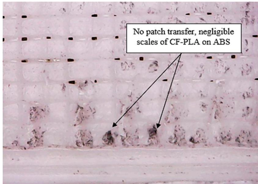
**Figure 6.** No patch transfer from the CF-PLA to ABS portion after delamination.
