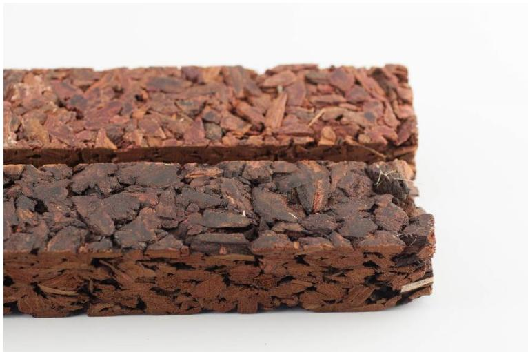
**Figure 1.** Larch bark insulation panel (glued with tannin in the foreground and UF in the background (thickness = 20 mm, density = 400 kg/m<sup>3</sup>).
