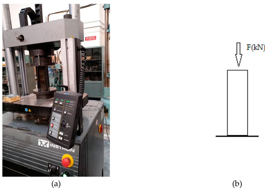
Figure 7. (a) INSTRON press of HTM-HYD 300 kN during the compression tests; (b) Representation of compression measurement.
