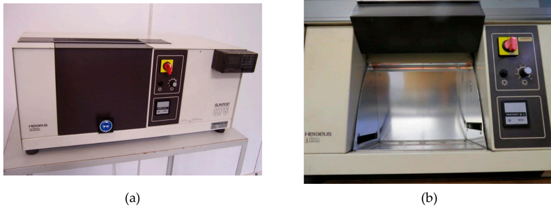
Figure 8. (a) SUNSET CPS ATLAS used for the artificial aging; (b) Booth where the specimens were exposed to UV radiation at 550 \text{ W/m}^2 (295–800 nm).
