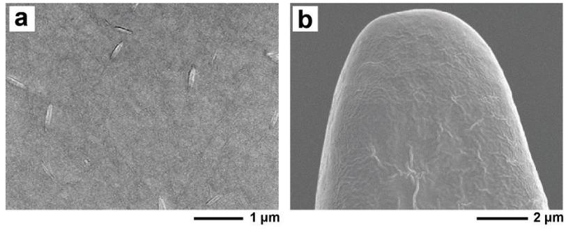
**Figure S1.** SEM images showing (a) the front side (needles were distributed) of the backing layer and (b) the needle surface of the SDMN patch.
