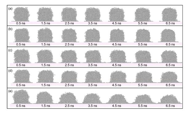
**Figure 3.** Snapshots of the spreading process of PP droplet with simulation time on the smooth surface. The temperature of PP droplet was (**a**) 383 K, (**b**) 413 K, (**c**) 443 K, (**d**) 473 K and (**e**) 503 K respectively.
