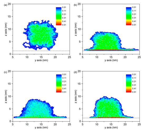
**Figure 7.** Density distributions of the PP droplet on different substrate. (**a**) initial density of PP droplet on Al substrate, final density distributions of PP droplet on (**b**) Al substrate, (**c**) Ni substrate and (**d**) Fe substrate at the simulation time of 6.5 ns.
