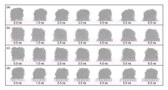
**Figure 5.** Snapshots of the spreading process of PP droplet with simulation time on Al substrate with rough surface. The side length of the column array was (**a**) 0.40 nm, (**b**) 0.64 nm, (**c**) 0.81 nm and (**d**) 1.21 nm respectively.
