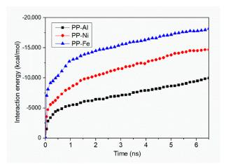
Figure 8. Interaction energies at PP-Al, PP-Ni and PP-Fe interface as a function of simulation time.
