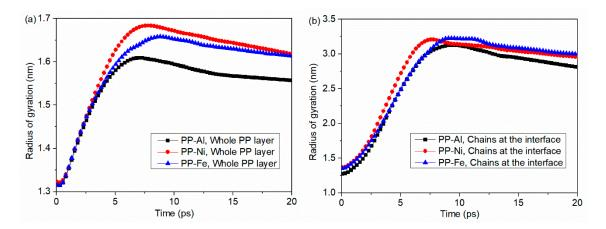
**Figure 10.** Radii of gyration in PP layer during the separation process with different substrate structures. The radius of gyration is calculated for (**a**) the whole PP layer and (**b**) molecular chains at the interface that are obviously stretched during the separation.
