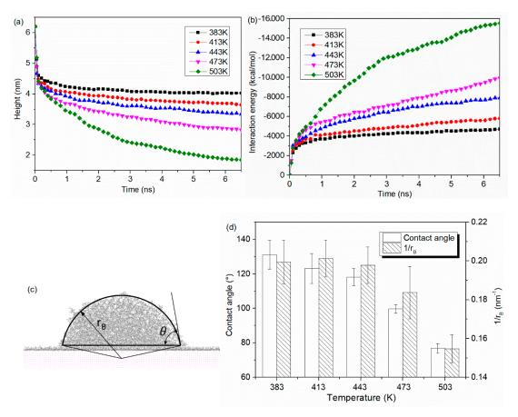
**Figure 4.** (a) height of mass center and (b) interaction energy as a function of simulation time, (c) calculation of contact angle and base radius and (d) contact angle and base radius of PP droplets on Al surface at different temperatures. The temperature of PP droplet was ranging from 383 K, 413 K, 443 K, 473 K to 503 K.
