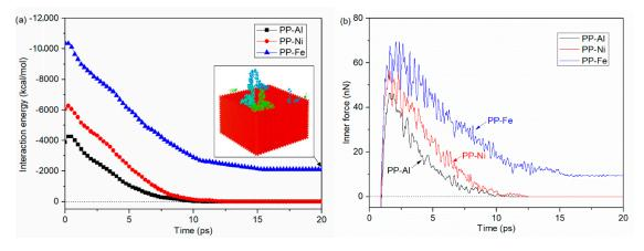
**Figure 11.** (**a**) interaction energies of injection-molded polymer-metal hybrid structure and (**b**) inner forces in PP layer during the separation process with different substrates.
