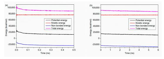
**Figure 2.** Energy distribution as a function of simulation time during (**a**) the first 0.5 ns and (**b**) the later 6.0 ns. The potential energy, kinetic energy, non-bonded energy and the total energy are calculated, respectively.
