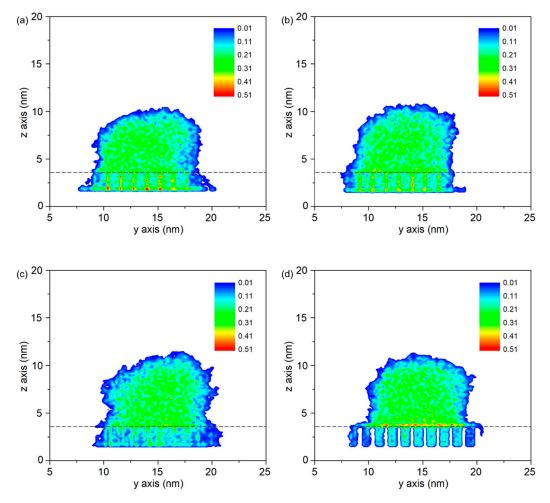
**Figure 6.** Density distributions of the PP droplets on Al substrate with different rough surfaces. (a) column arrays with side length of 0.40 nm (P1), (b) column arrays with side length of 0.64 nm (P2), (c) column arrays with side length of 0.81 nm (P3) and (d) column arrays with side length of 1.21 nm (P4).
