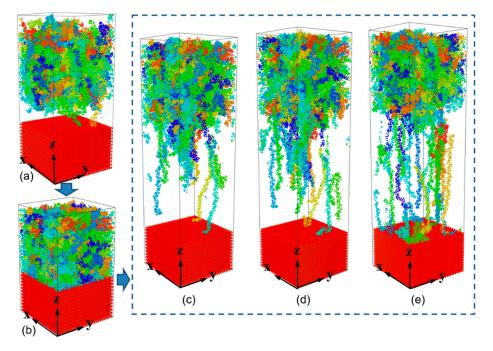
**Figure 9.** Snapshots of PP-metal hybrid structure during the injection molding and separation process. (a) the original PP-metal layer is constructed and then (b) injection-molded to form a hybrid system. After cooling process, an external force was applied to remove the PP layer away from the metal substrate. These snapshots are taken at a separation time of 10 ps, with the substrates of (c) Al, (d) Ni and (e) Fe, respectively.
