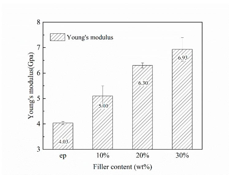
Figure S4 Young's modulus for epoxy and HF-Ti<sub>3</sub>C<sub>2</sub>T<sub>x</sub>/epoxy composites
