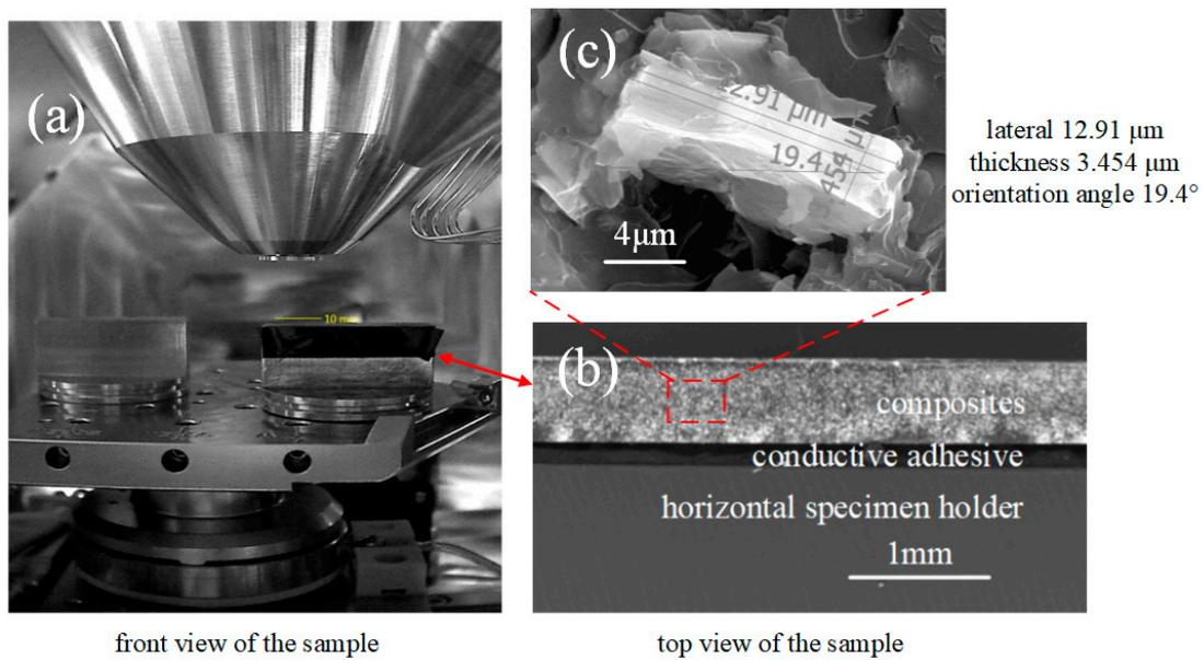
Figure S2. Demonstration of estimating orientation angle using SEM
