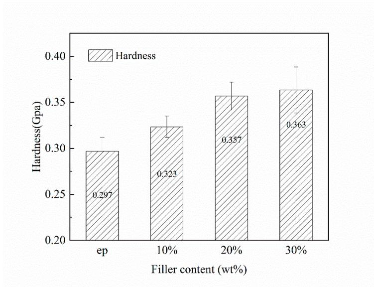
Figure S5 Hardness for epoxy and HF-Ti<sub>3</sub>C<sub>2</sub>T<sub>x</sub>/epoxy composites
