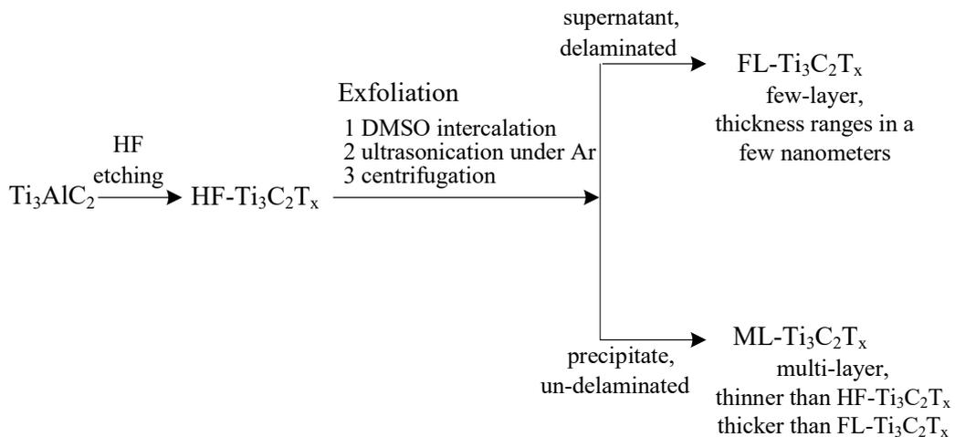
Figure S1. The process of manufacturing three forms of  $\text{Ti}_3\text{C}_2\text{T}_x$
