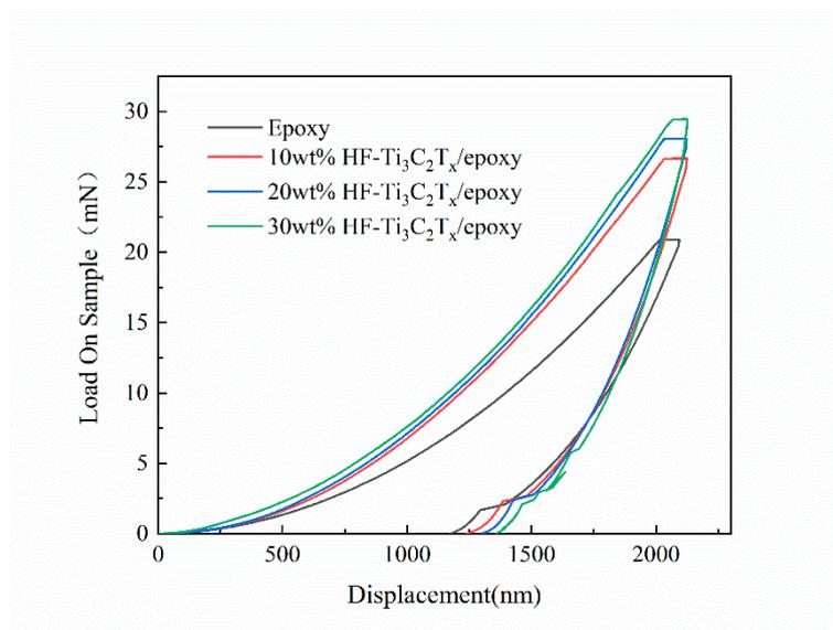
Figure S3 Load-displacement results in nanoindentation tests
