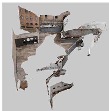
**Figure 5.** Digital model B' obtained with terrestrial photogrammetry.
