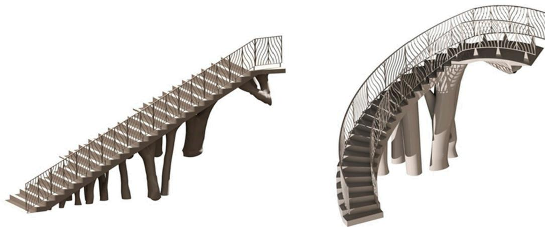
**Figure 29.** Geometrical models of the construction elements under study, imported into the BIM environment  $E_1$  (left) and  $E_2$  (right).
