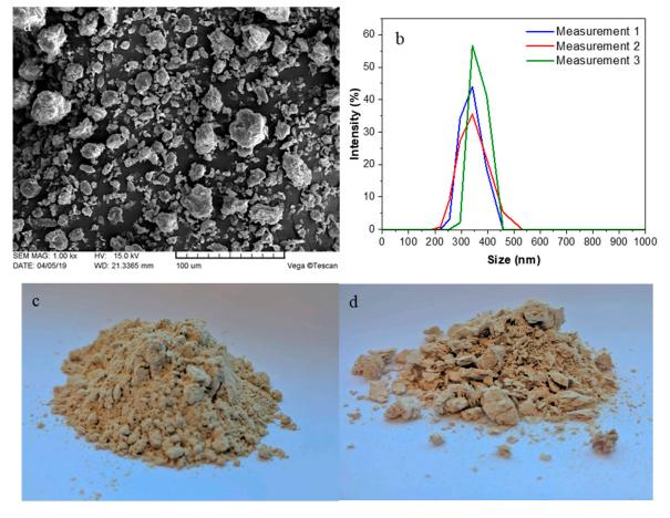
**Figure 1.** (a) Scanning electron microscopy micrograph of microcrystalline cellulose (MCC); (b) dynamic light scattering analysis of nanofibrillated cellulose (NFC); (c) dry MCC filler and (d) freeze-dried NFC filler.
