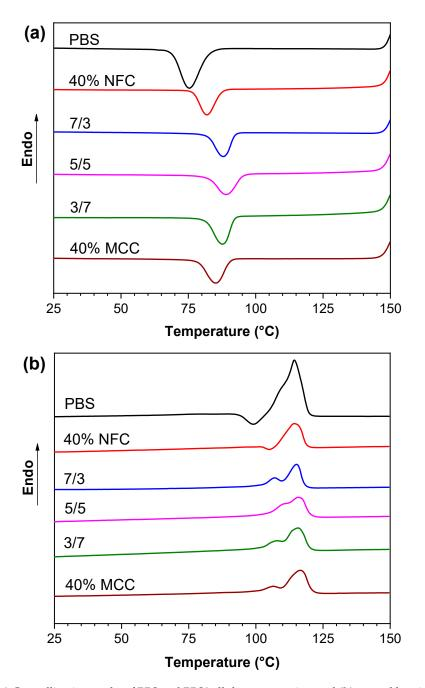
**Figure 3.** (a) Crystallization peaks of PBS and PBS/cellulose composites and (b) second heating melting peaks of PBS and PBS/cellulose composites under the nitrogen atmosphere.
