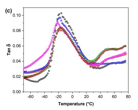
**Figure 4.** (a) The storage modulus E'; (b) the loss modulus E'' and (c) loss tangent tan  $\delta$  curves of PBS and PBS/cellulose composites.
