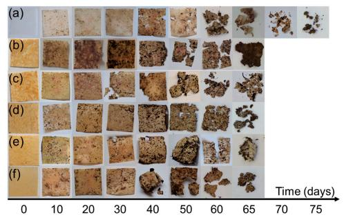
**Figure 8.** Photos of (**a**) PBS; (**b**) 40% NFC; (**c**) 7/3; (**d**) 5/5; (**e**) 3/7 and (**f**) 40% MCC films during biodegradation studies in soil burial test conducted in composting conditions.
