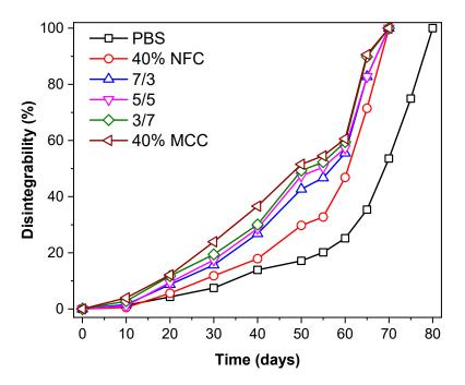
**Figure 7.** Percentage weight loss of PBS and PBS/cellulose composites in soil burial test conducted in composting conditions.
