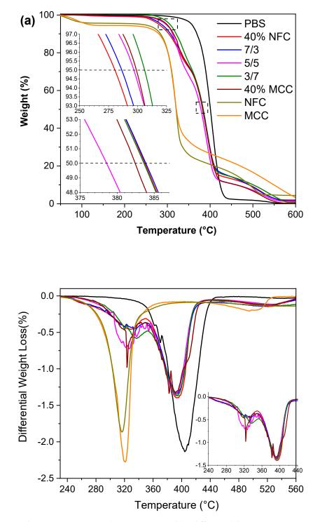
**Figure 2.** (a) Thermogravimetric analyses contours and (b) differential thermogravimetric contours of PBS, PBS/cellulose composites, NFC and MCC under air atmosphere.
