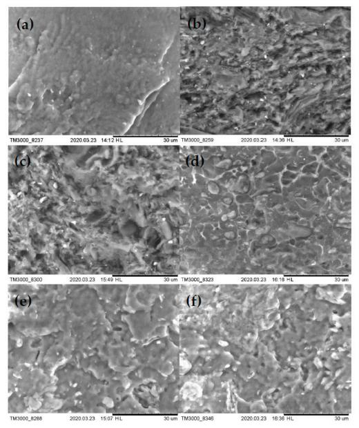
**Figure 6.** Scanning electron microscopy micrographs: (**a**) PBS; (**b**) 40% NFC; (**c**) 7/3; (**d**) 5/5; (**e**) 3/7 and (**f**) 40% MCC.
