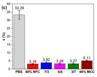
**Figure 5.** Tensile strength results of PBS and PBS/cellulose composites: (**a**) Elastic modulus E; (**b**) tensile strength  $\sigma$  and (**c**) strain  $\varepsilon$ .
