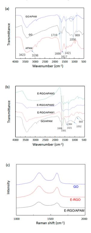
**Figure 2.** (a) FT-IR spectrum of APAM, GO, GO/APAM; (b) FT-IR spectrum of E-RGO/APAM with ethylenediamine dosage of (1–3) 0.1, 0.5, 1.0 mL, respectively; (c) Raman scattering spectrum of GO, E-RGO, E-RGO/APAM.
