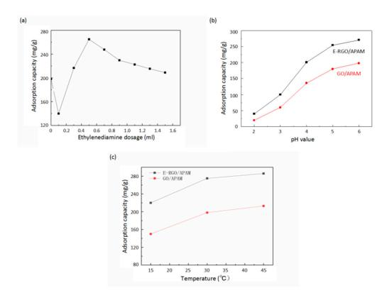
**Figure 4.** (a) Effect of ethylenediamine dosage on adsorption capacity of E-RGO/APAM; (b) effect of pH value on adsorption capacity of GO/APAM and E-RGO/APAM; (c) effect of temperature on adsorption capacity of GO/APAM and E-RGO/APAM.
