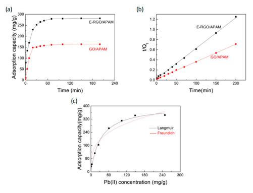
**Figure 5.** (a) Influence of adsorption time on the adsorption capacity of GO/APAM and E-RGO/APAM; (b) pseudo second order kinetic equation fitting of Pb(II) adsorption by GO/APAM and E-RGO/APAM; (c) Langmuir and Freundlich adsorption model of E-RGO/APAM (conditions: pH = 5, T = 30 °C).
