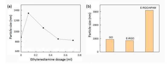
**Figure 1.** (a) ethylene diamine-reduced graphene oxide (E-RGO) particle size of different ethylenediamine dosage; (b) particle size of graphene oxide (GO), E-RGO and ethylene diamine-reduced graphene oxide/anionic polyacrylamide (E-RGO/APAM).
