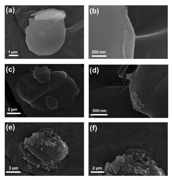
**Figure S1**. FE-SEM images of BNPDA with various input ratio of BN and DA (a, b) 1:0.2, (c, d) 1:0.4, and (e, f) 1:0.8.
