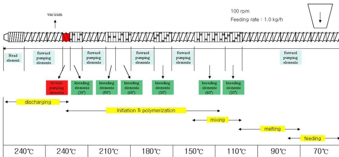
Figure S2. Screw configuration and barrel temperature.
