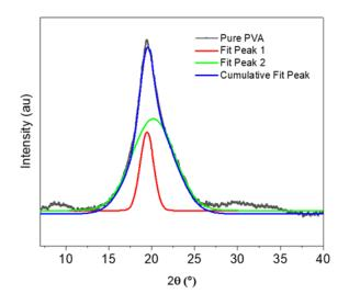
Figure S1. The deconvolution of XRD patterns of pure PVA film
